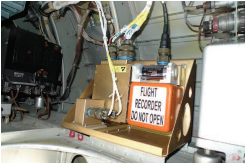
Flight Data Recorder installation
