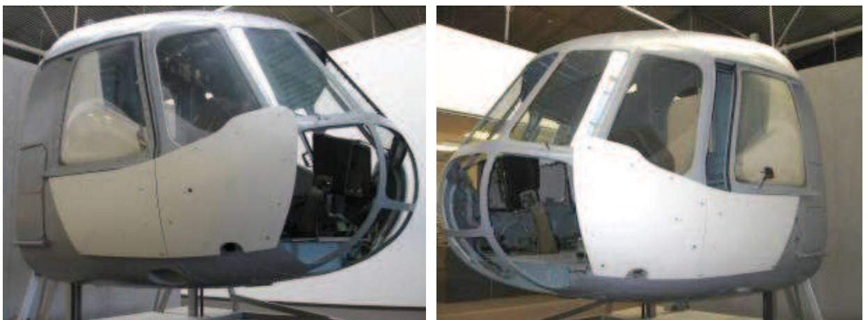
Fig.2 Outside ceramic composite panels installed
